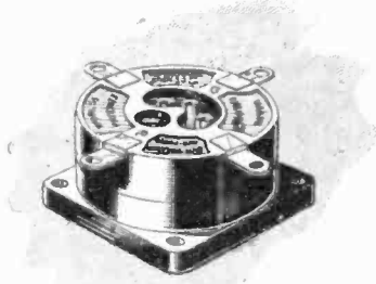
The sockets of the Artic valve holder are suspended by means of gauze strips, the wire strands of the gauze being arranged obliquely to minimise the transmission of microphonic noises between the socket and the Bakelite mounting piece.
