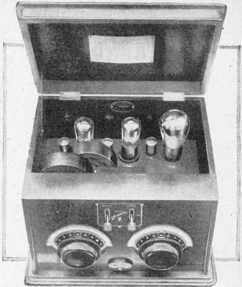
The interior of the set presents a particularly clean appearance. Note the tuning chart inside the lid and engraved resistance sockets and valve holders.
